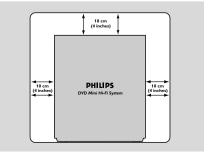
The ventilation should not be impeded by covering the ventilation openings with items, such as newspapers table-cloths, curtains, etc.
